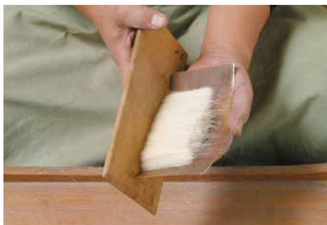
“Brush kneading” is performed at the tip of each brush by craftsmen.
