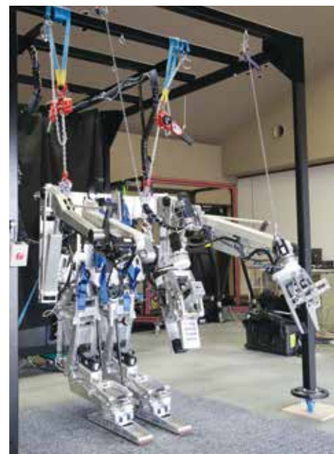
POWERLOADER "NIO" (Research material aiming to fully use in nuclear plant and disaster relief)
