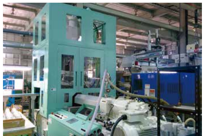
Blow molding machine performing integrated production by the hot parison method
