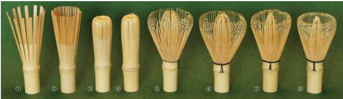
①Thinning down ② Fine splitting ③ Thinning and stroking ④ Chamfering ⑤ Lower braiding ⑥ Upper braid ⑦ Alignment ⑧ Finishing
